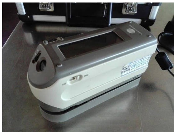
Figura 6: colorimetro KONICA MINOLTA CM-2500d
